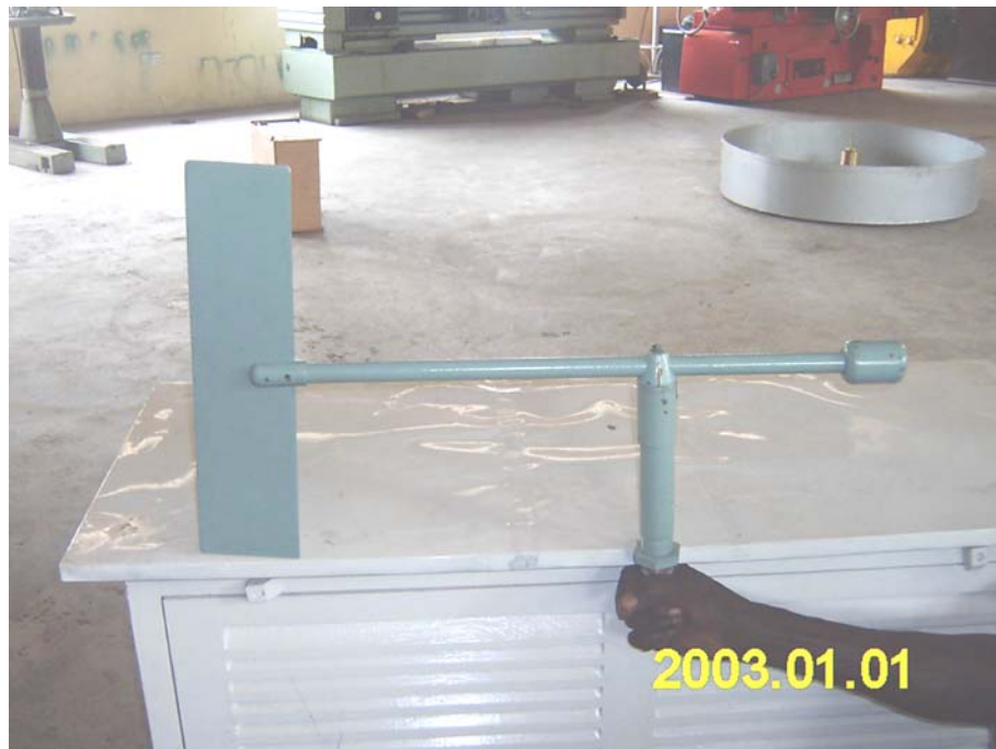
Fig. 4.0 Wind vane produced at the workshop
