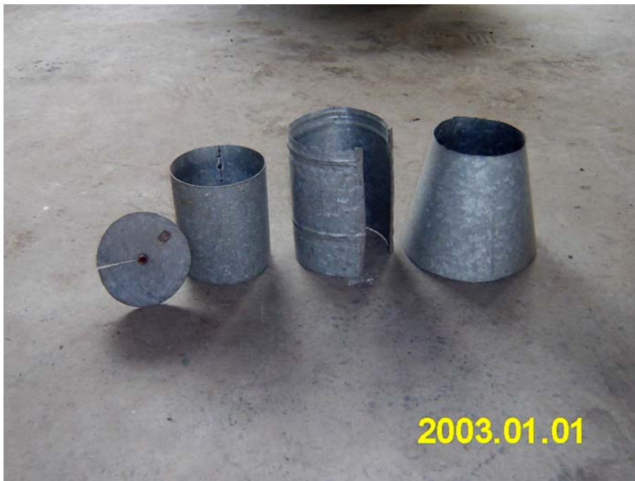
Fig. 5.0 Production process of a simple rain gauge
