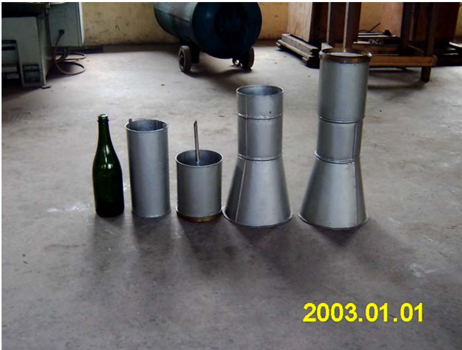
Fig. 6.0 Component parts of a simple rain gauge
