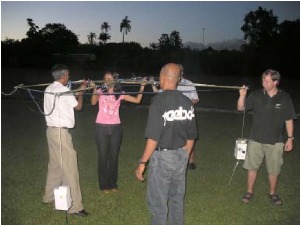
Fig.1 Graw and Sippican 3 thermistor radiosondes ready for a night time comparison of the Vaisala-Sippican-Graw radiosonde group on the bamboo cross support rig.
