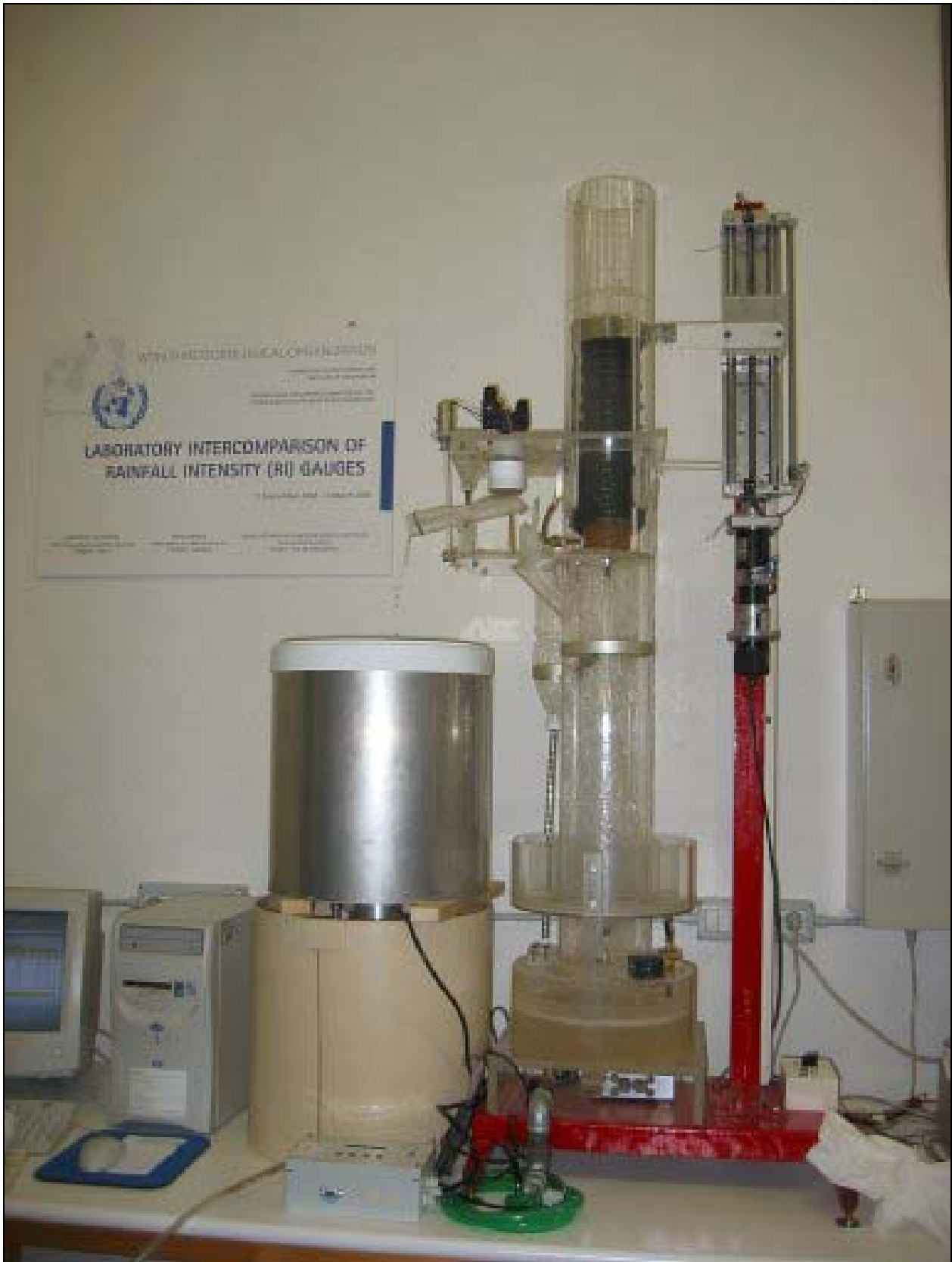
Figure 2: A tipping-bucket rain gage under test at the laboratory of DIAM (University of Genoa).
