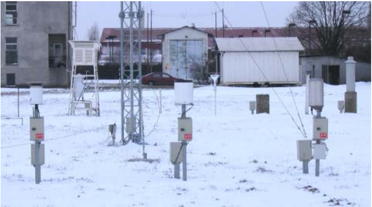
Figure 1. Tested rain gauges at meteorological observatory Zagreb – Maksimir
