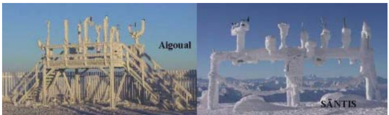
Fig. 2: Test platforms with different sensors at Mont Aigoual (left) and Säntis (right)
