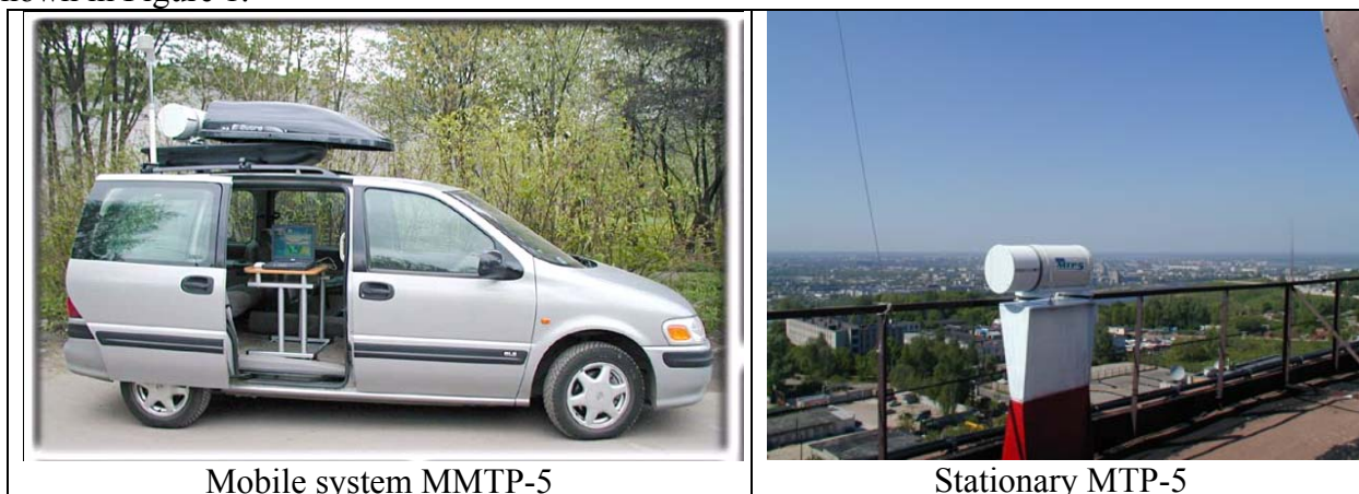
Fig. 1. Common view of temperature profilers.
