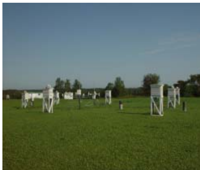
Figure 5 - General view of temperature/humidity sensors installation in CARE test site.
