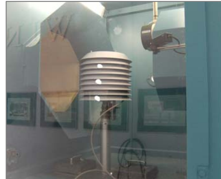
Figure 4. Setup of the KNMI screen in the wind tunnel where the response time was estimated by cooling the screen starting at roughly 45°C.
