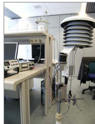
Figure 1. Setup of the air flow experiment conducted on the LAM630 screen.
