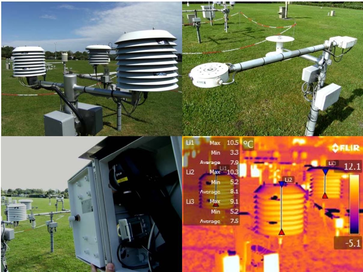
Figure 7. Instrumentation used in the field trial. The upper panels present: (left) the KNMI aspirated screen, the LAM630 screen and the KNMI standard screen with clearly visible the thermistors fitted to the lamellas and (right) the instrument setup for total and shortwave upward and downward radiation. The bottom panels show: (left) the camera enclosure with its contents and (right) an example of the FLIR thermal image pointed at the three main screens under study, presenting the minimum and maximum temperatures for selected areas.
