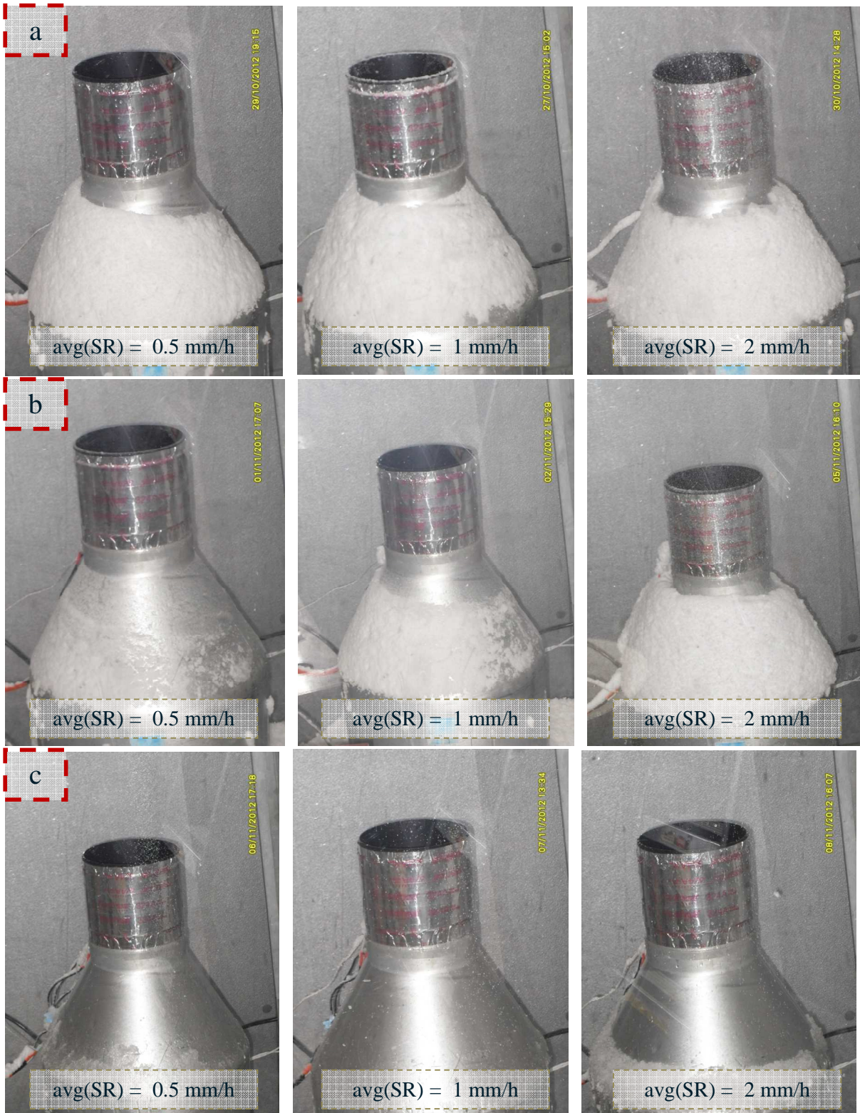
Fig. 6: Snow accumulation of the GEONOR T200B case after 1 mm of equivalent water. The gauge was equipped with an internal and an external AC heater stripe (100W)
