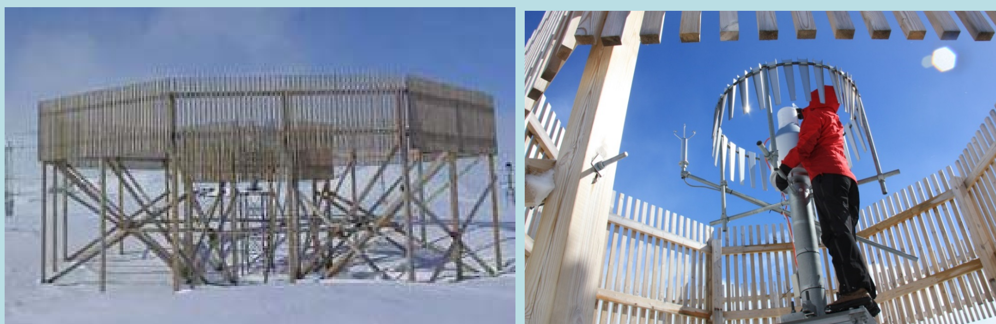
This Double Fence Intercomparison Reference (DFIR), specified by WMO-SPICE is minimizing the wind-effect on the precipitation measurements, allowing to measure the (almost) true precipitation and the calculation of the catch-ratio for the standard gauge outside.
