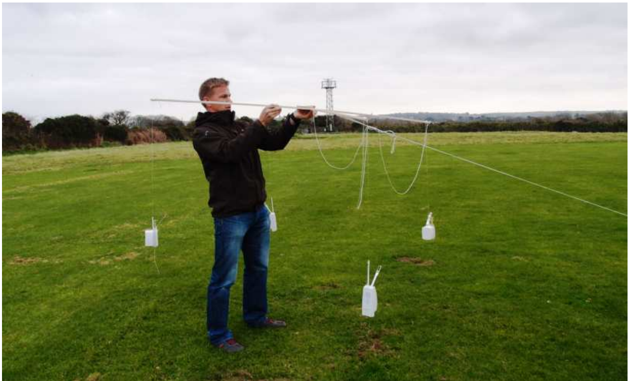
Figure 8. Test flight rig in Camborne test campaign with two RS41 and two RS92 Radiosondes
