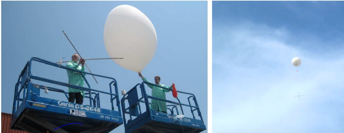
Figure 18. Preparing the four-radiosonde test rig release in Penang, Malaysia
