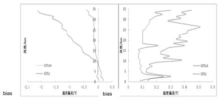
The atmospheric long-wave radiation correction in nighttime was the main consideration. But for smaller bead temperature sensor, if the surface is aluminized coating, the impact of atmospheric long-wave radiation cannot basically been considered.
