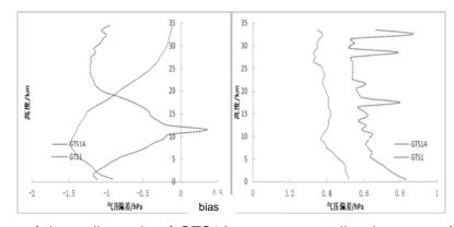
The pressure of the radiosonde of GTS1A type was smaller than one of RS92 type. The standard deviation was within 0.5hPa. It was less than the radiosonde of GTS1 type. The stability was better than the radiosonde of GTS1 type.
