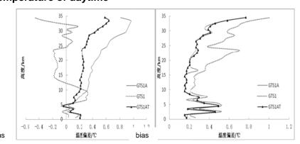
In daytime, solar radiation effect on temperature was the main consideration. In addition to surface coating, the most important thing is the radiation correction algorithm. The casting data in  $4\text{th} \sim 9\text{th}$  September 2010 was statistically analyzed.
