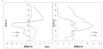
Compared to the radiosonde of RS92 type, the system error and standard deviation of humidity of the radiosonde of GTS1A type were smaller than ones of the radiosonde of GTS1 type.
