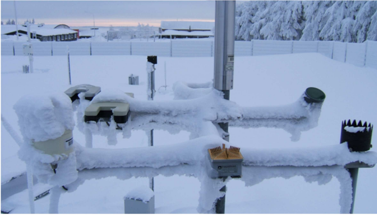
Figure 8: Field set up at Wasserkuppe after heavy snow fall. Snow is accumulated at the wind shields of the precipitation sensors while the heating is not sufficient.
