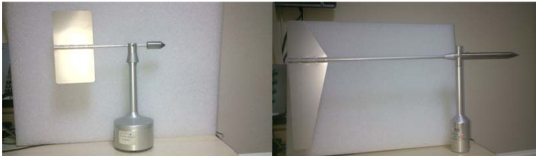
Figure 1-b: Images from wind direction sensors.
