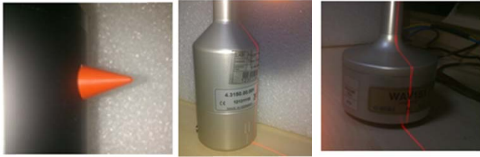
Figure 2: Images of north cursor of different wind direction sensor models.
