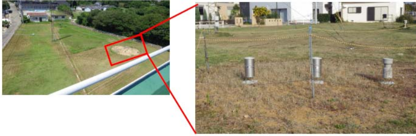
Fig.1 Installation of rain gauges at the test field(left), 1.0mm type (left), 0.5mm type(center) and 0.2mm type(right).
