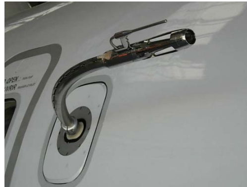
Figure 5 : Condensation Particle Counter, on the ATR42-SAFIRE plane , allowing the detection and the counting of particles by enlarging them, using the particles as nucleation centers to create droplets
