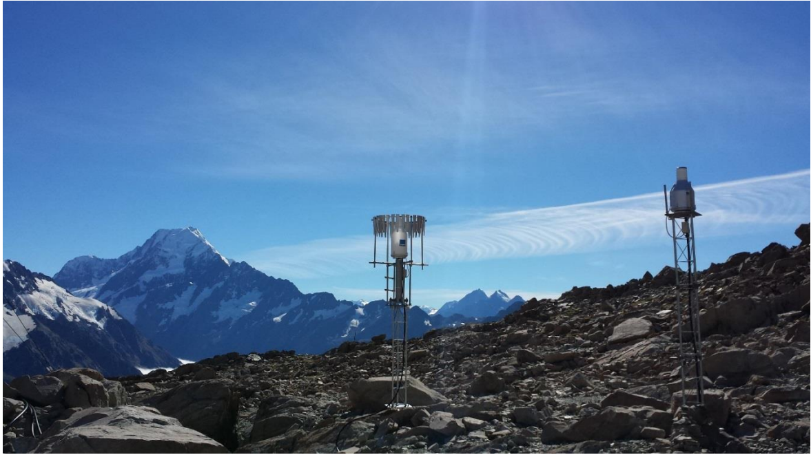
Figure 6: Layout of the Geonor gauges on site. The G1 gauge with alter shied is in the centre of the image with the un-shielded G2 gauge to the right of the photo. Note both gauges atop the lattice masts (rims 4.1m above ground level). Aoraki/Mt Cook is in the background, to the left of the picture.
