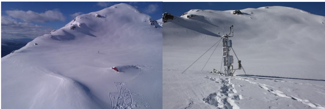
Figure 5: Deep snow pack taken 23 October 2012. Snow depth sensor appeared to have malfunctioned until a site visit revealed that it was buried under snow.
