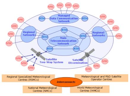
Figure 1. High-level schematic of the Global Telecommunication System (GTS) (source: http://www.wmo.int/pages/prog/www/TEM/GTS/index\_en.html)
