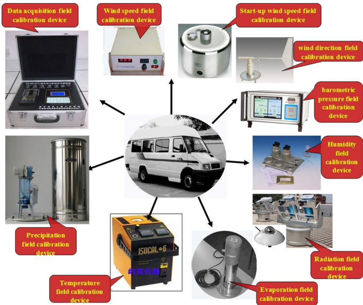
Fig 9 Mobile field meteorological calibration system
