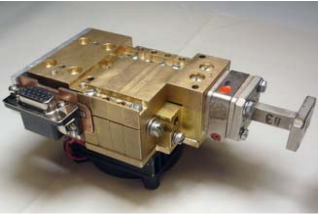
Figure 4 Microwave receiver with isolator
