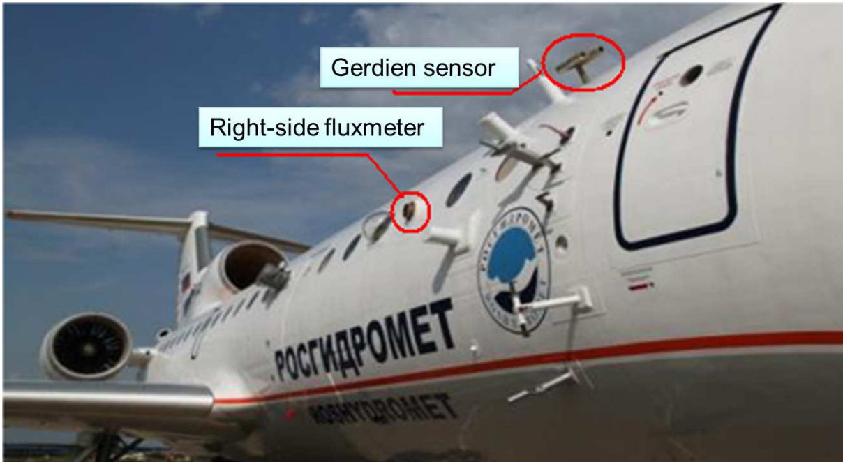
Figure 4. The aircraft sensors installation.
