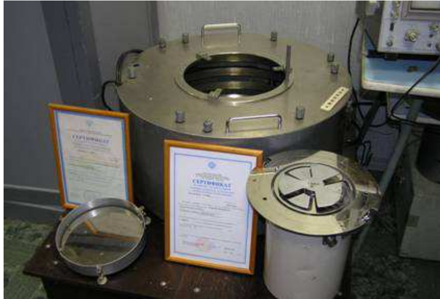
Figure 7. Electrical field strength calibrator (on background) and state certificate of correspondence (foreground).
