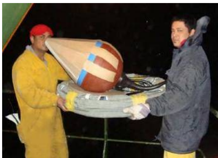
Figure 20. Deployment of the standard SVP-B drifter by means of drop to water
