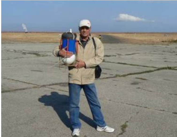
Figure 28. View of micro ice marker, equipped with parachute system to be deployed on ice or snow
