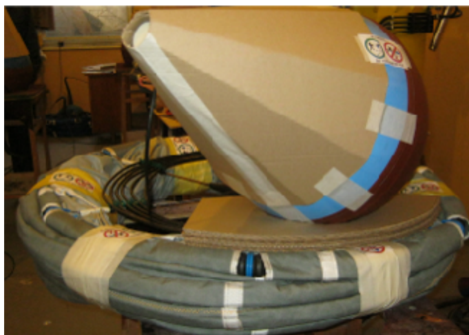
Figure 19. Main view of standard SVP-B drifter with 41-cm float and 92-cm drogue, prepared to be ready for self-deployment after drop to water
