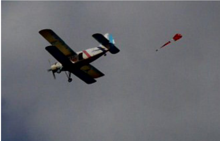
Figure 30. Opening of parachute after drop from aircraft
