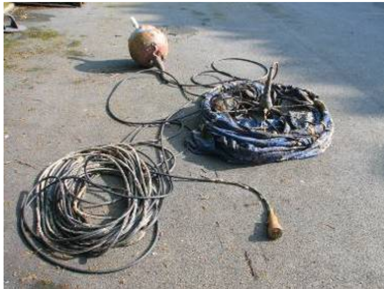
Figure 8. Main view of the SVP-BTC temperature-profiling drifter, which was recovered after one year operation in the Bay of Biscay
