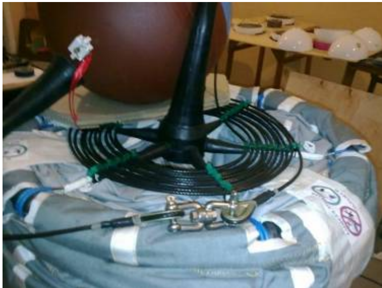
Figure 11. Spiral packaging of tether line in the clips, fixed to radials of “wire connection” and swivel, inserted in tether below float, to decrease probability of loops creation on tether during submergence of drogue after drop of buoy to water and influence of float’s bidirectional rotation on tether
