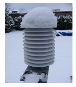
18 months several prototypes have been successfully tested, the subject of our research is now to prove to be able to demonstrate an accurate temperature recording in the range of 1/100 °C.
