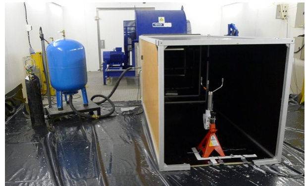
Figure 2. Test set-up includes water tank (blue), radial blower, air channel, water spraying nozzles, and UUT inside climate cabinet.
