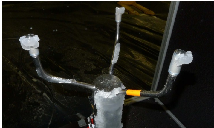
Figure 7. UUT after icing period. Translucent ice formed on surfaces facing wind. UUT was providing data.
