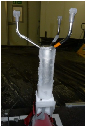
Figure 6. UUT after icing period. Ice layer on non-heated structure was 12 mm, while sensor tube has an ice cover of 8 mm.
