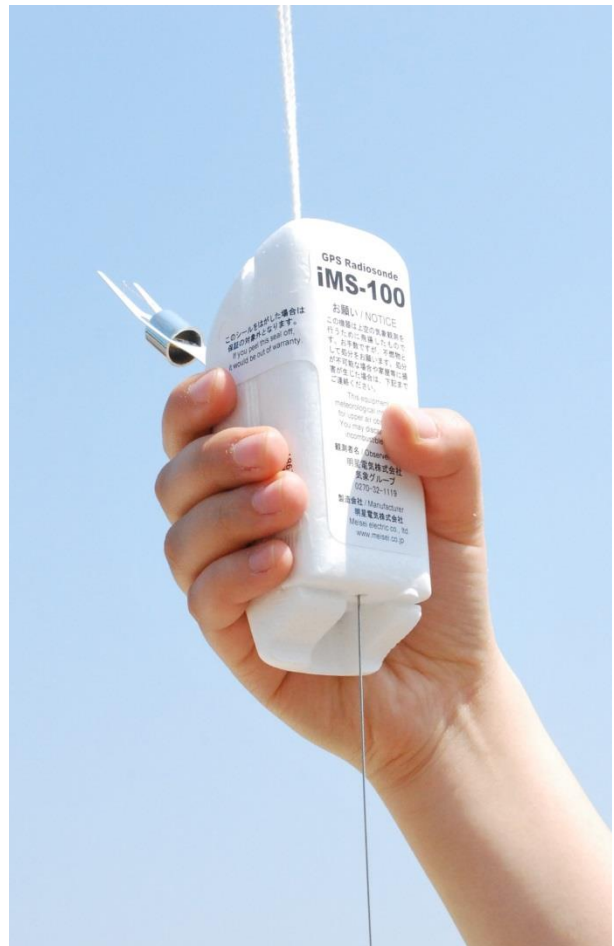
Figure 1: Outlook of micro sonde iMS-100
