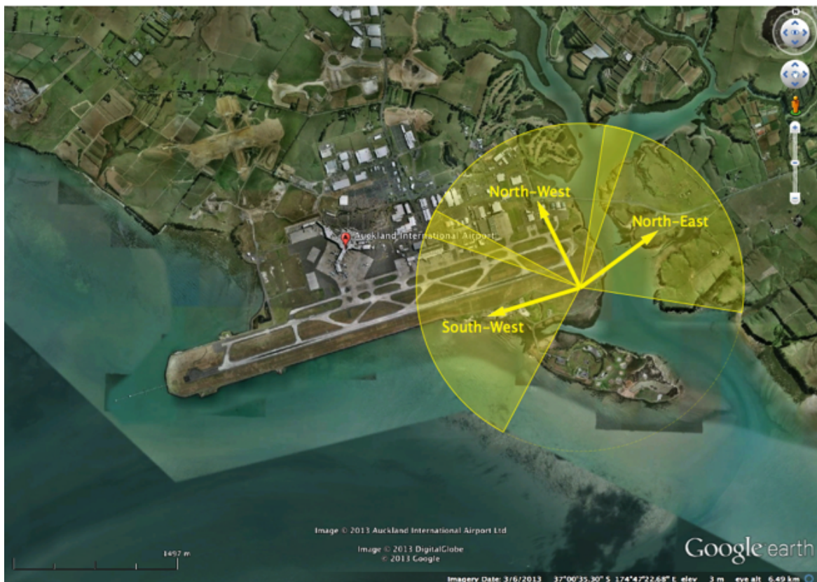
Example of Web camera alignment and coverage
