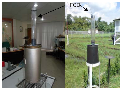
Figure 4. The Field Calibration Device (FCD)
