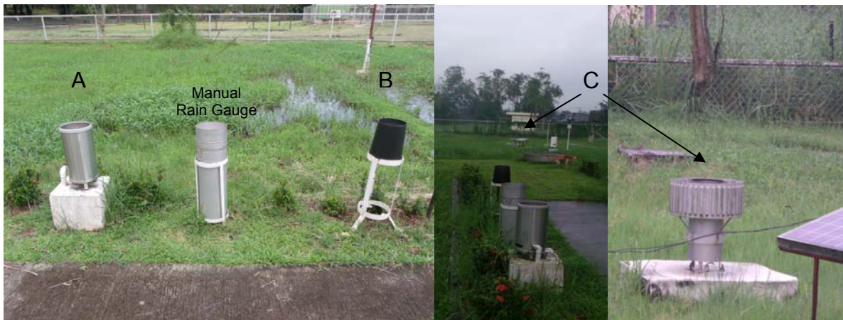
Figure 3. The manual rain gauge with the three (3) tipping buckets (A), (B), and (C)
