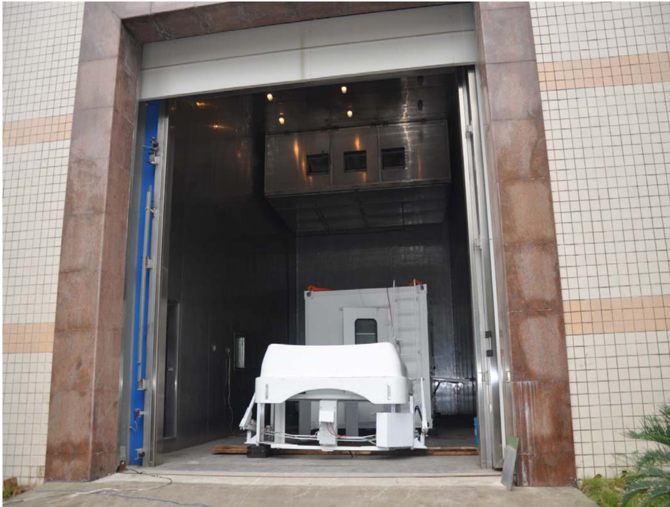
Fig. 6 High and Low Temperature Test of Remote Location Unattended upper-air sounding system
