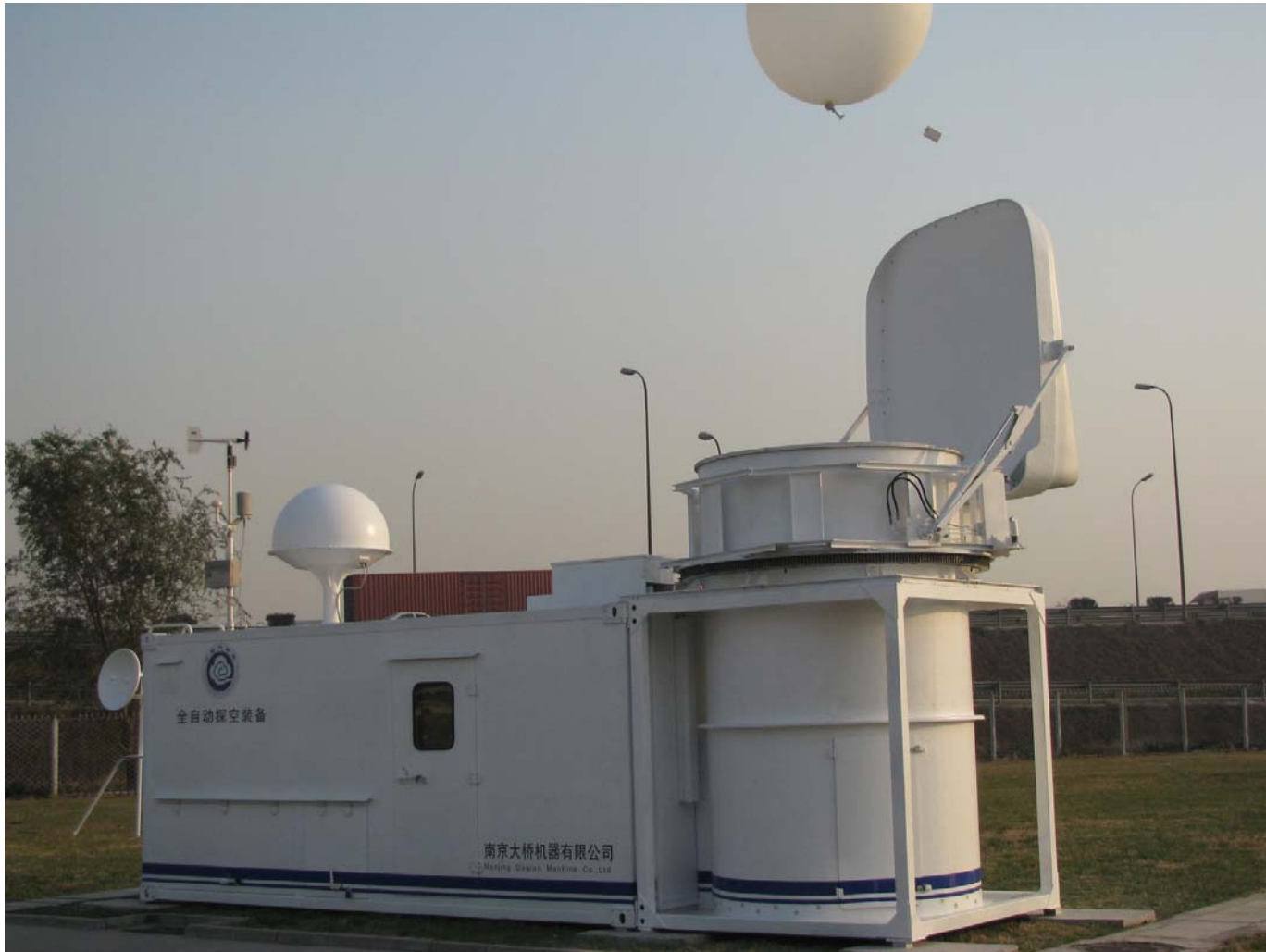
Fig. 1 Remote Location Unattended Station of Automated Sounding System
