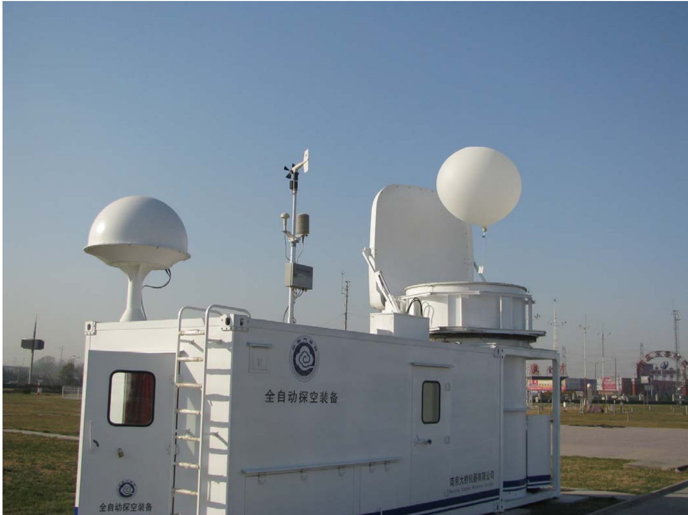
Fig. 2 Remote Location Unattended Station of Automated Sounding System
