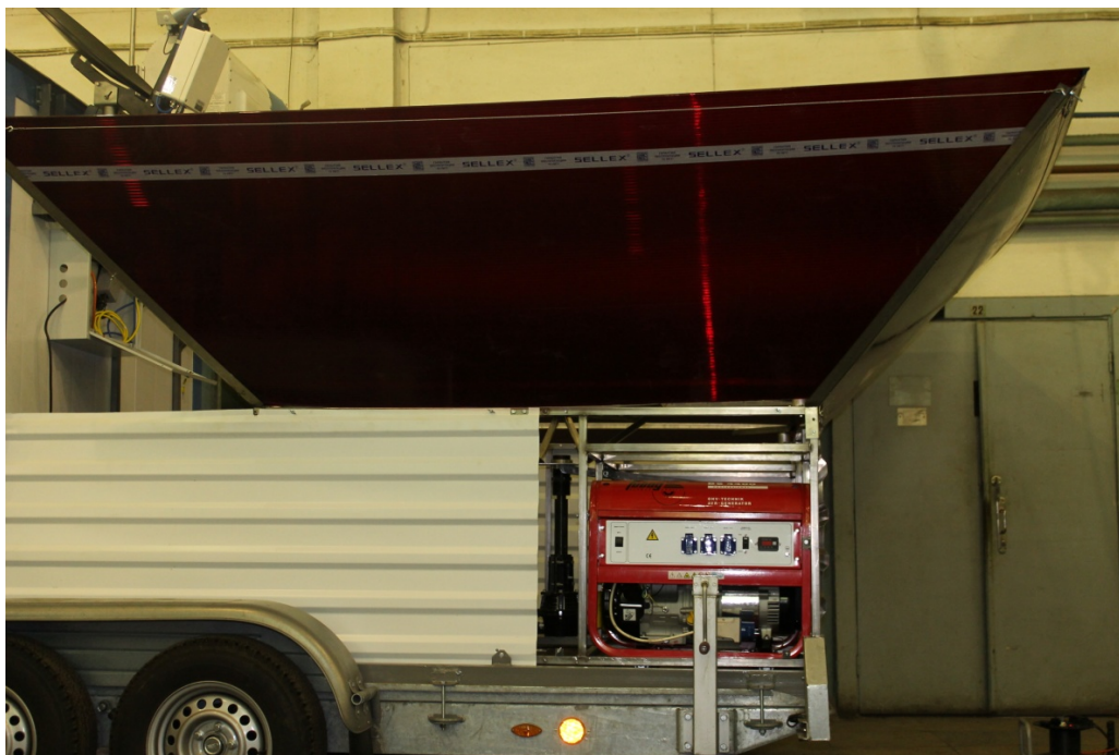
Figure 2 General view of the radar wind profiler with side lobes suppression screens
