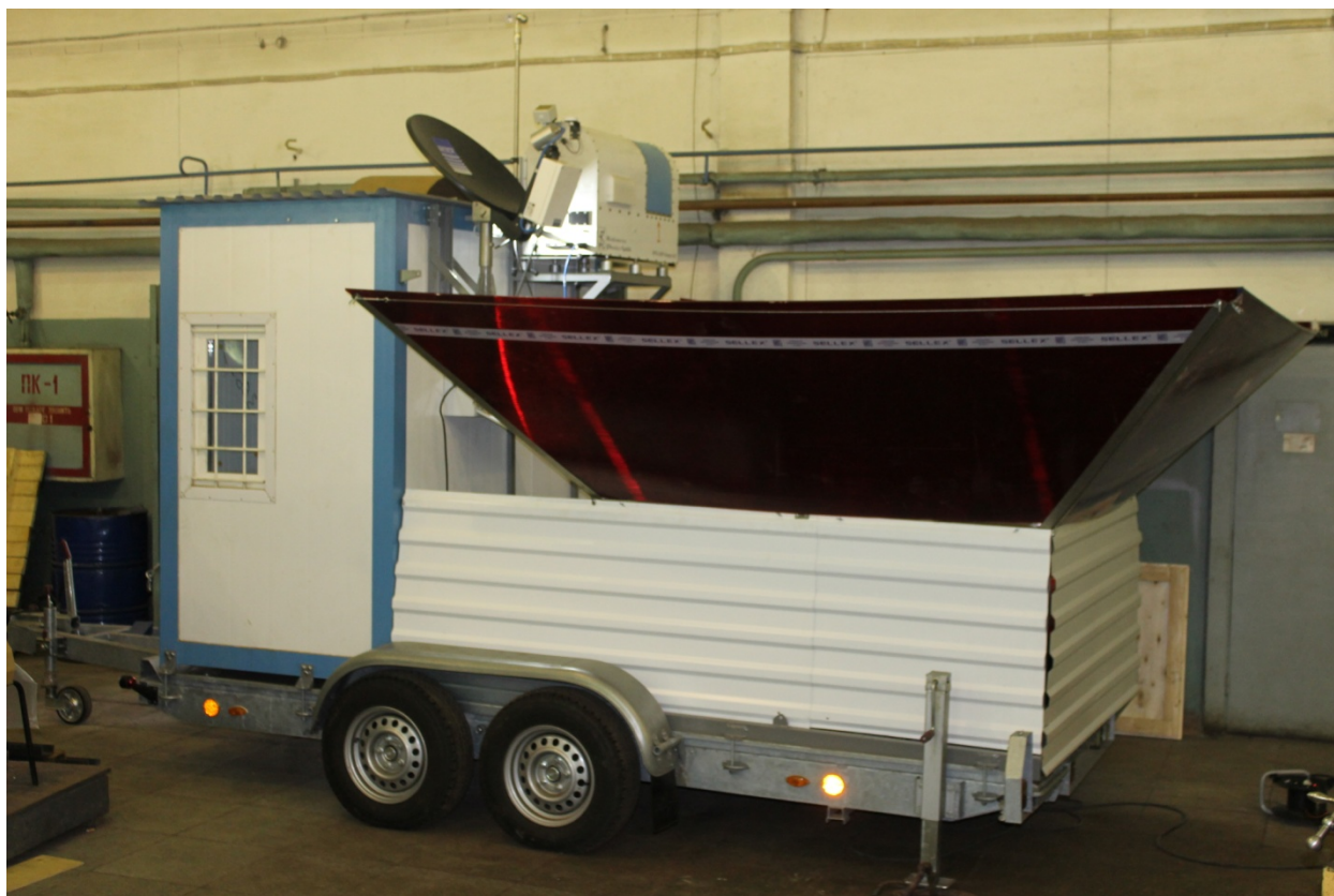
Figure 1. The general view of Mobile System for Atmosphere Remote Sensing
