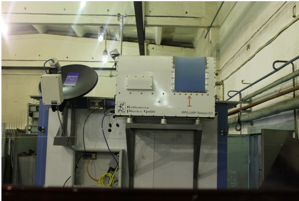
Figure 3 General view of the microwave temperature\humidity profiler (right) and Micro Rain Radar (left)
