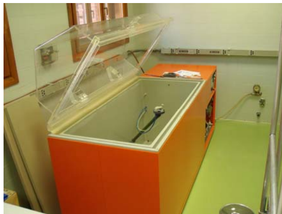
Figure 3. CEM salinity chamber
