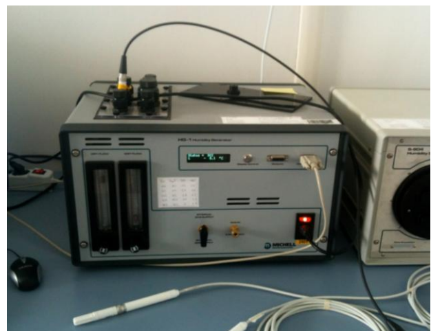
Fig. 5.1 Measures on different set points to adjust sensors' output (Michell HG-1 "chilled mirror").
