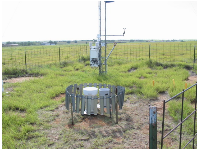
Figure 3. Site photo of the Mesonet continuity station in Beaver, Oklahoma. Both the current rain gauge and a heated gauge are deployed in the alter screen. Additionally, both a naturally ventilated and an aspirated temperature sensor are installed on the tower at 1.5 m.
