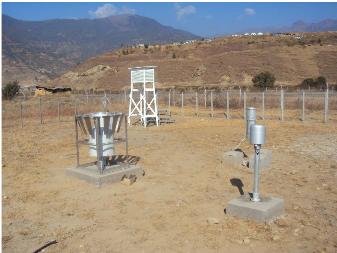
Fig.2. Department of Hydrology and Meteorology, Nepal, meteorological station at Jumla airport. The LTB (Right), OP2W (left) and manual raingauge and stevenson screen (behind)
