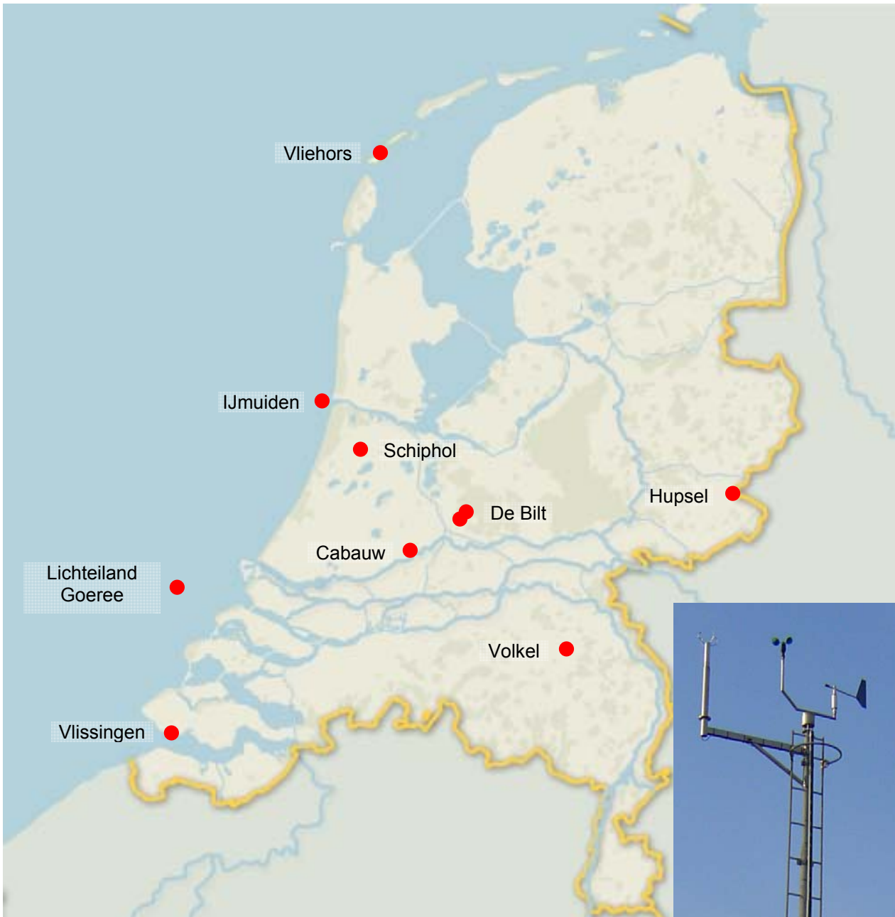
Figure 7: The locations of the operational test of ten Thies 2D sonics in the Netherlands. The inset shows the parallel field setup with the sonic and the operational cup anemometer and wind vane.
