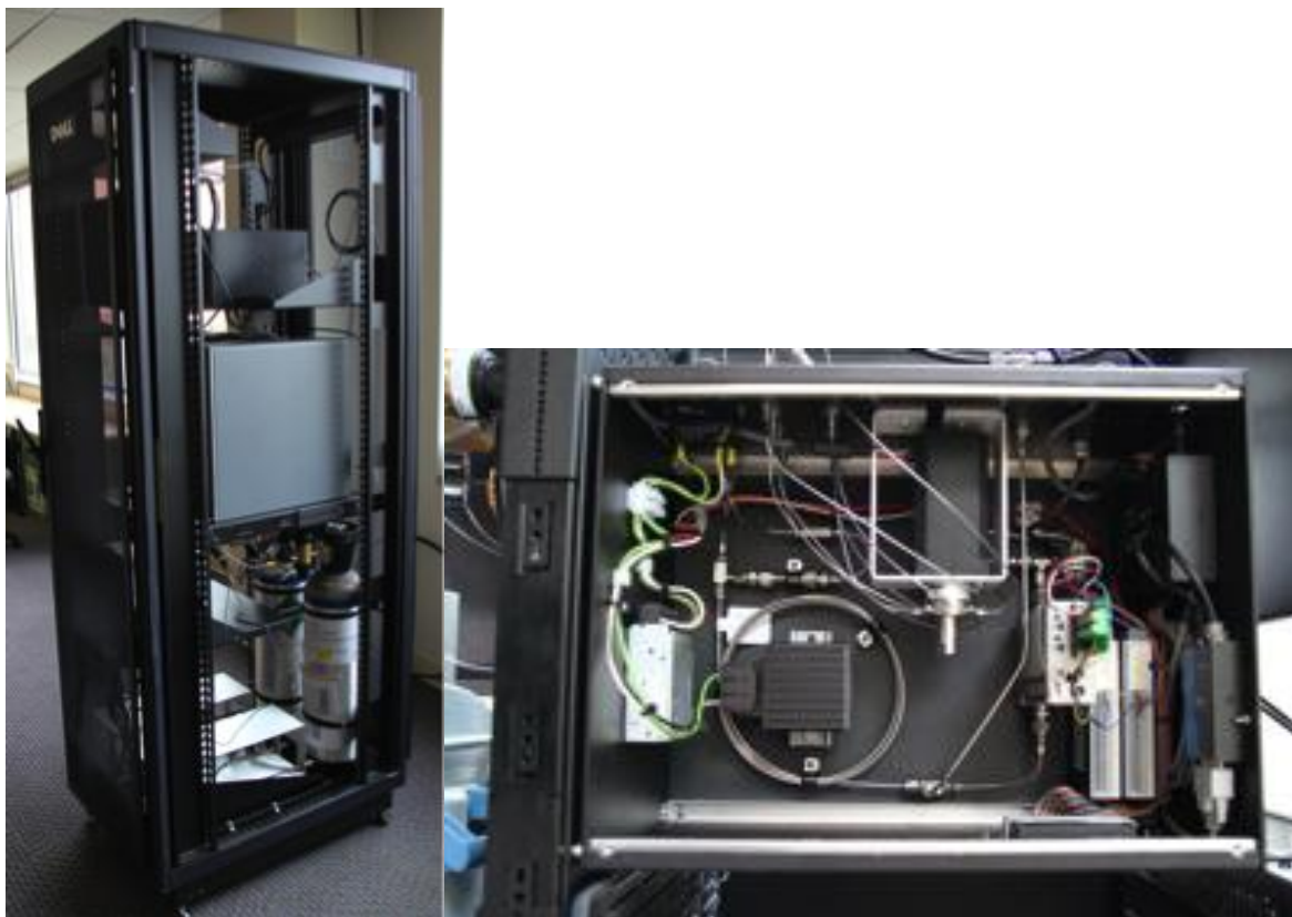
Figure 3. Earth Networks sampling and calibration system.
