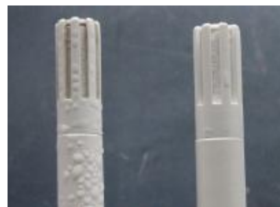
Figure 10: Two HMP 155 sensors after 3 hours of high humidity conditions during the laboratory test. The HMP155 sensor on the right is heated, the one on the left is unheated.
