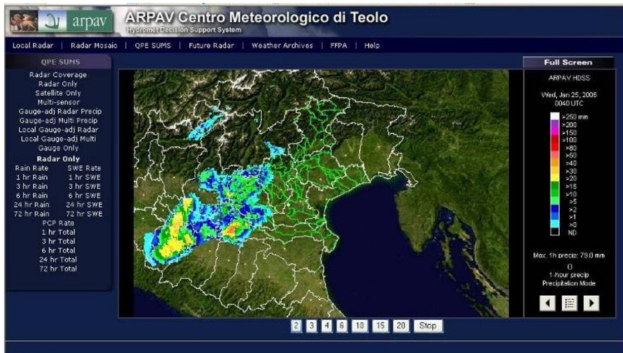
Figure 12. Example of rain estimates for a one hour time frame from QPEA. Green lines show the basin delineation over the region.
