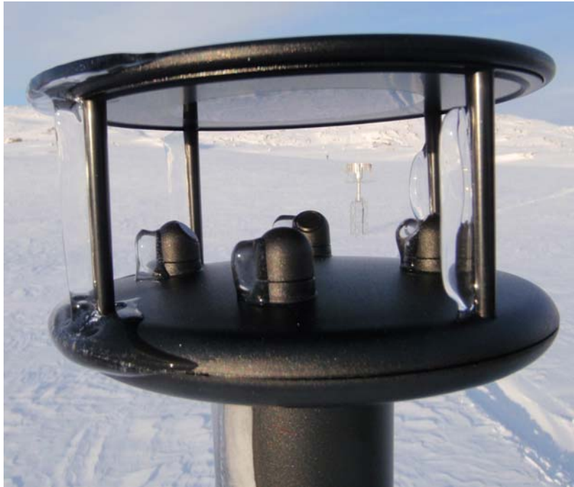
Figure 12: Gill WindSonic with icing. Data from this test site is not included in this study.
