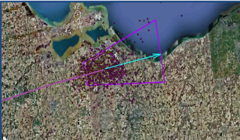
Figure 6: An alert polygon can be created for the area 45 minutes ahead of the moving cell.
