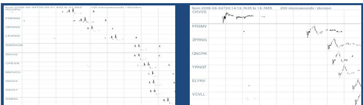
Figure 1: The graph on the left shows the waveforms from an IC pulse, across multiple sensors in WTLN. The graph on the right shows the waveforms from a return stroke (CG).
