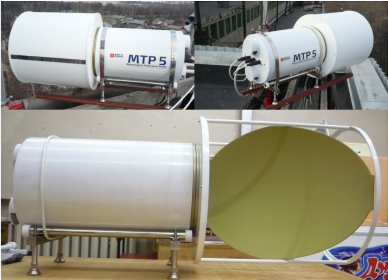
Fig. 4 General overview of MTP-5PE and photo of antenna system.
