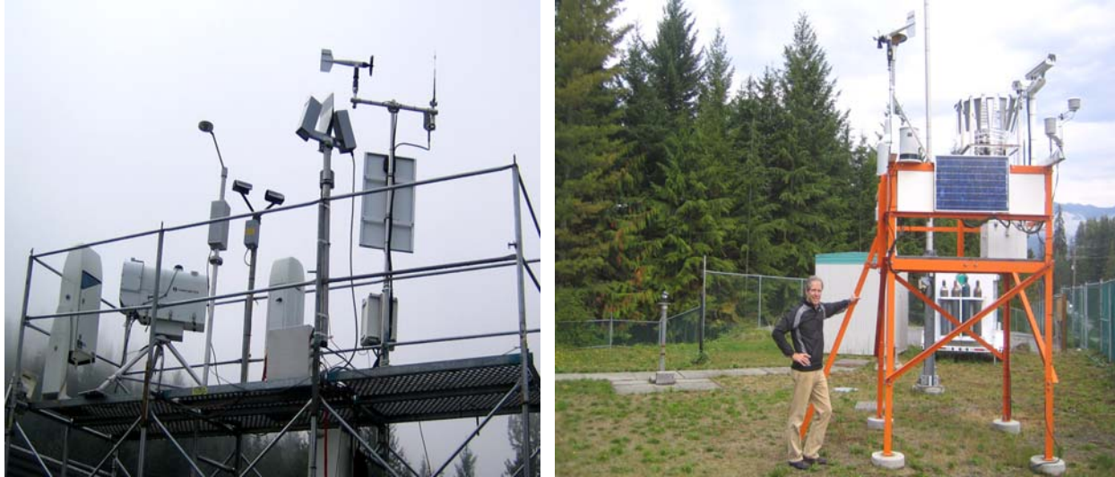
Figure 2. Meteorological sensors (radiometer second from left) on the mountainside at the base of the Creekside Gondola, and the radiosonde launch site in the Whistler valley.
