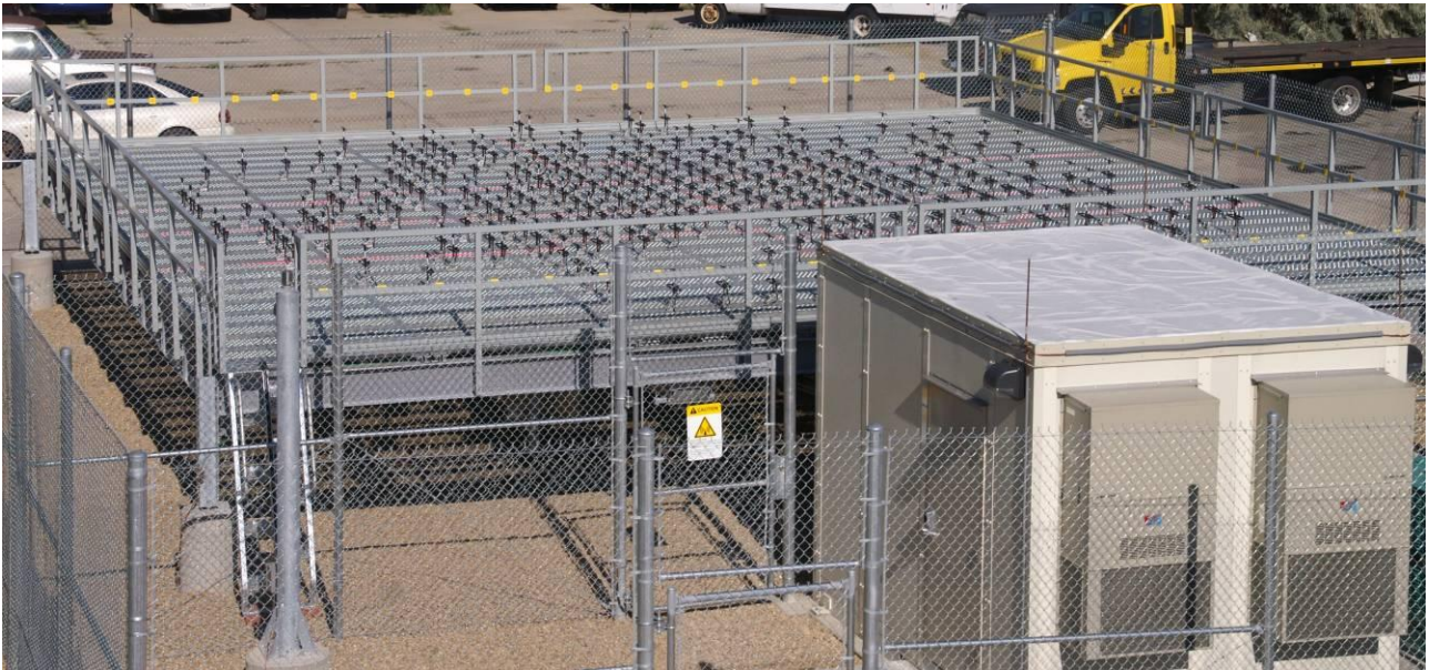
Figure 1: DeTect, Inc. RAPTOR FBS-ST radar wind profiler. This picture shows the NOAA NWS demonstration unit produced and installed in Longmont, Colorado, USA.
