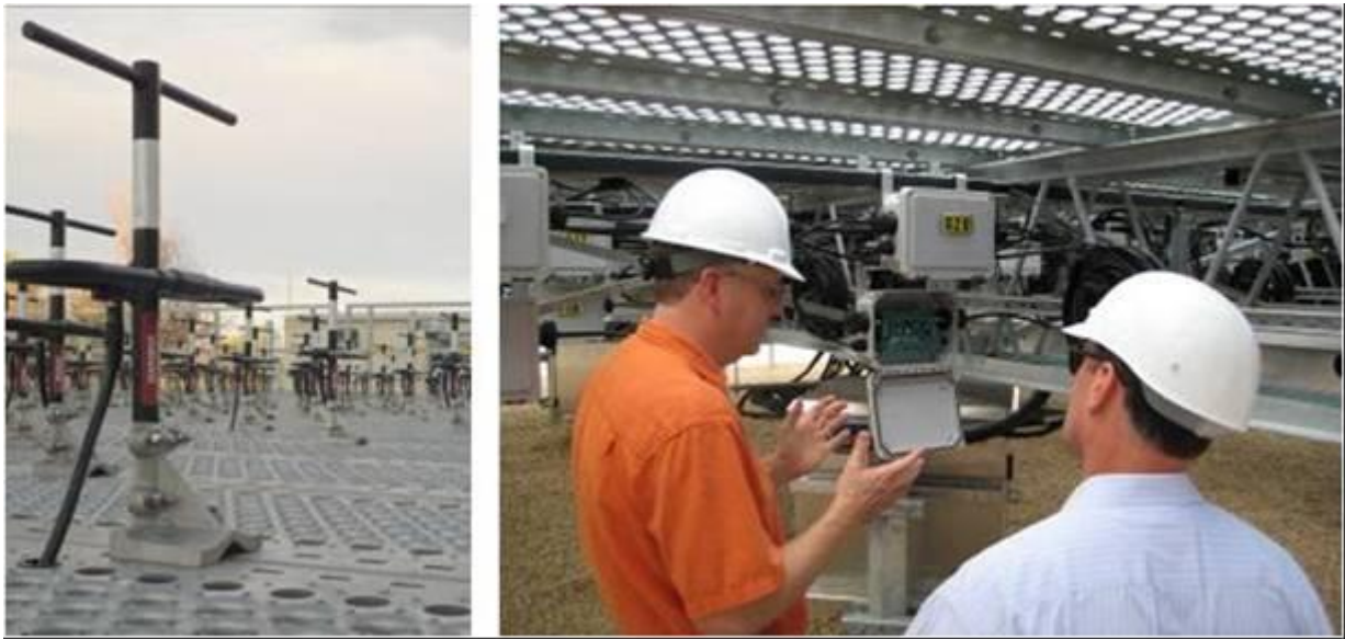
Figure 2: Top side of antenna array (left) and underside of array (right). Underside picture shows the solid-state phase shifters.
