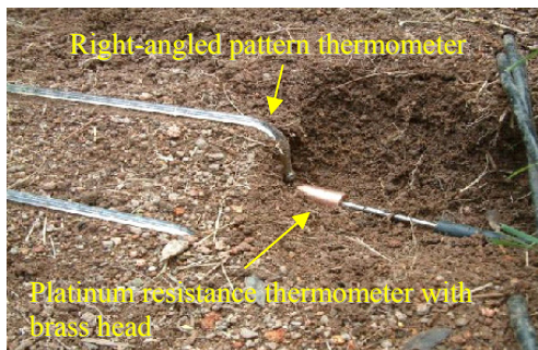
Figure 2. Angled pattern earth thermometer (Cassella) installed next to a platinum resistance thermometer for shallow depth soil temperature measurement.
