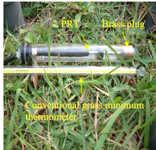
Figure 4. Sheathed PRT for the grass temperature alongside the conventional grass minimum thermometer. The brass plug inside the glass sheath was removed in final the operational system.
