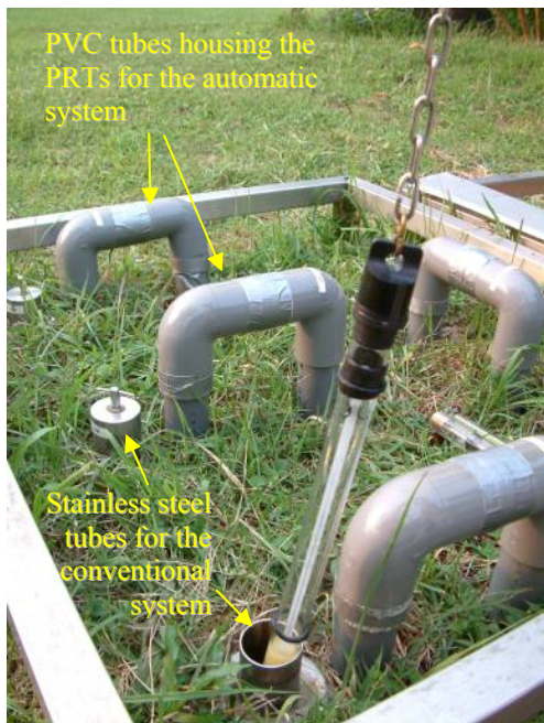
Figure 3. 50 cm depth sheath pattern earth thermometer (Cassella) extracted from its stainless steel tube for measurement. The grey PVC tubes next to the conventional thermometers houses the individual PRT thermometers of the automated system for each depth.
