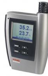
Temperature and humidity readout equipment for monitoring atmospheric condition at the calibrating laboratory
