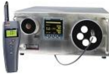
Humidity generator (ROTRONIC- HYGROGEN-2)
