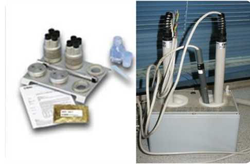
mirror chilled humidity standard and calibrating set based on fixed point solution
