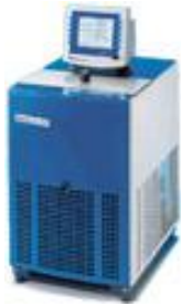
Liquid bath for temperature (WIKA-CTB 9400)
