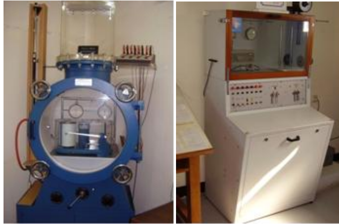
Existing pressure and humidity test chambers
