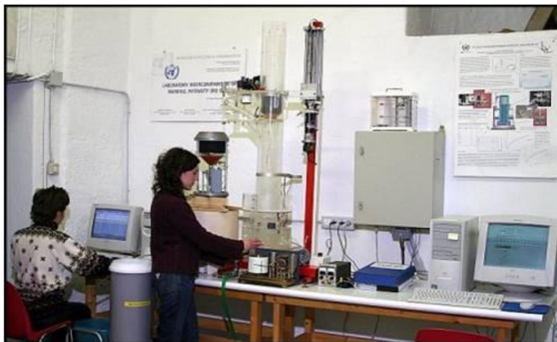
Fig. 4: The Qualification Module for Rainfall Intensity Measurement Instruments developed at the University of Genova, and used in the laboratory calibrations.
