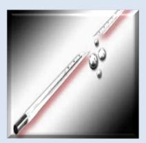
Despite great care in their handling, mercury barometers and thermometers can break, and although the pieces may be cleaned up in a timely manner, it is common that the mercury from these instruments can ball up and escape into small cracks or concealed places. It can also cling to objects such as brooms or shoes, and so swiftly spread from one place to another. Undetected mercury vaporizes and can be inhaled by those nearby, thus entering their bloodstream.
