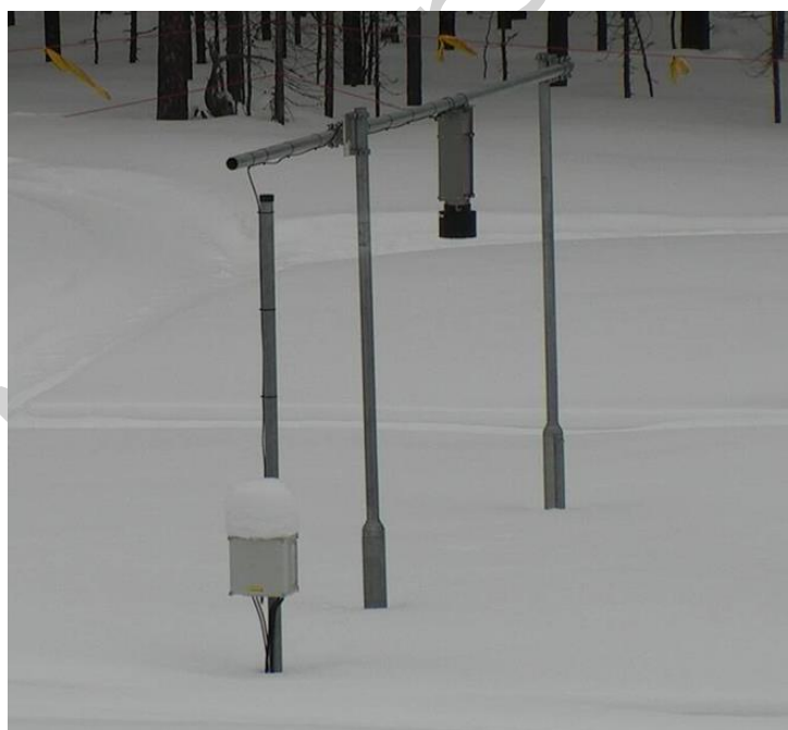
Figure 2.18. Passive gamma radiation SWE instrument (courtesy of FMI).
