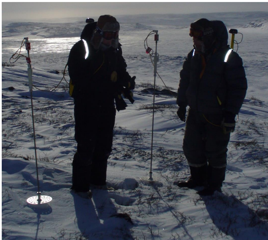
Figure 2.5. Self-recording GPS equipped snow depth probe in use (Canadian Arctic; photo courtesy of Environment and Climate Change Canada).
