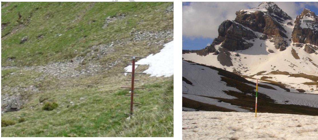
Figure 2.3. Vertical snow stakes with horizontal cross arms (left, photo courtesy of SLF) and colour coded bands (right, photo courtesy of AEMET).
