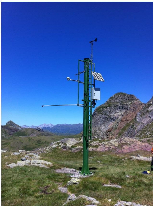
Figure 2.9. Sonic snow depth instrument (Pyrenees of Spain, photo courtesy AEMET)
