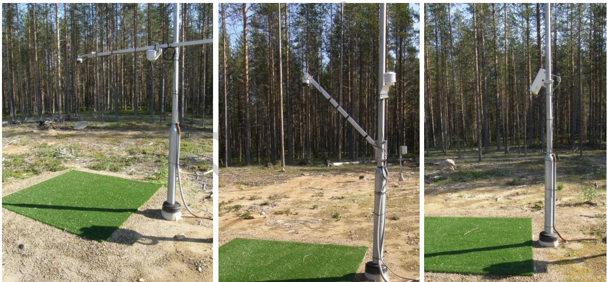
Figure 2.8. Automated sonic snow depth instrument mounting with steel mounting beam and pole secured with concrete (left), angled mounting beam to reduce collection of snow (middle), and laser instrument mounted at an angle away from the vertical mounting pole (right). (Photos courtesy of FMI, Sodankylä).
