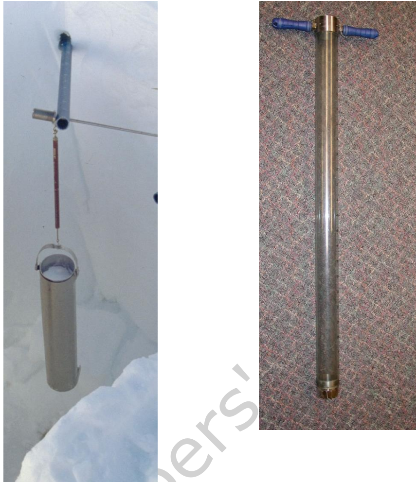
Figure 2.13 A volumetric sampler (left, 55 cm in height; courtesy of SLF) being weighed with a spring scale and a tube snow sampler (right; courtesy of Environment and Climate Change Canada).
