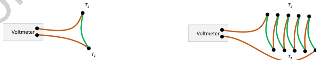
Figure 2.8. Use of thermocouple in differential mode: (a) difference between the two junctions (b) 'thermo pile'
