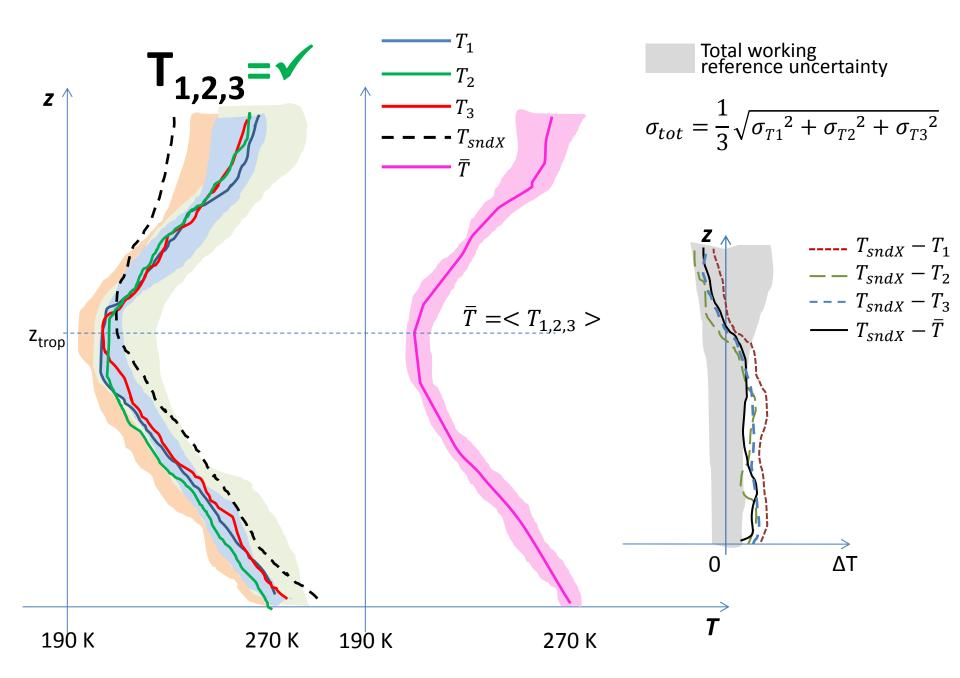
For a specific flight: working reference 3 is <u>rejected</u> based on the consistency condition
