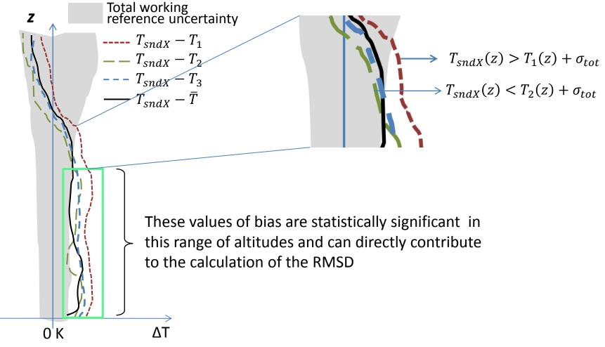
At the end of the intercomparison, after N flights, the total root mean square deviation (RMSD) of each sonde versus each working reference is calculated for those altitudes where  $|\Delta T| > \sigma_{tot}$
