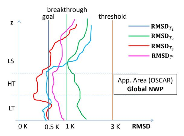
Each RMSD profile is calculated, potentially, from a different number of points for each level z. This is due to the fact that the sonde sndX at level z can have a statistically significant bias with respect to one working reference but not with the other.
