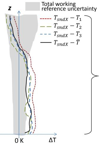
All data are retained despite the fact that the bias is statistically significant or not. Then, all  $\Delta T(z)$ points from all flights contribute to the RMSD. The final mean bias corresponds then to an average of the  $\Delta T(z)$  for all z-levels and all flights
