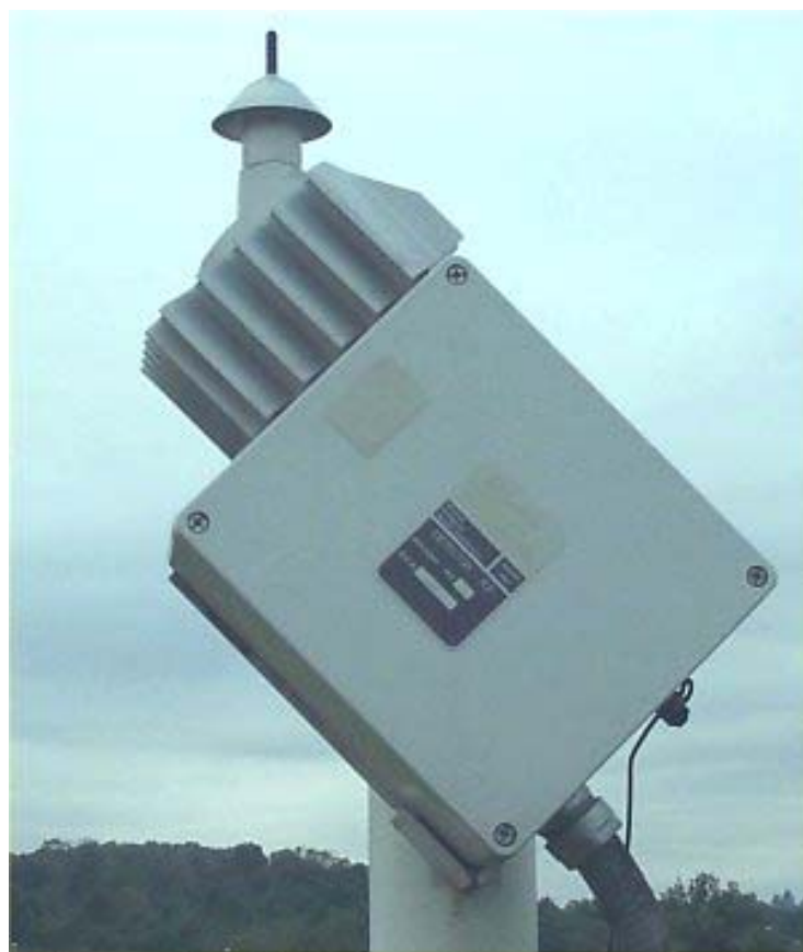
Figure A. 22 The Rosemount freezing rain sensor mounted at an AWOS site
