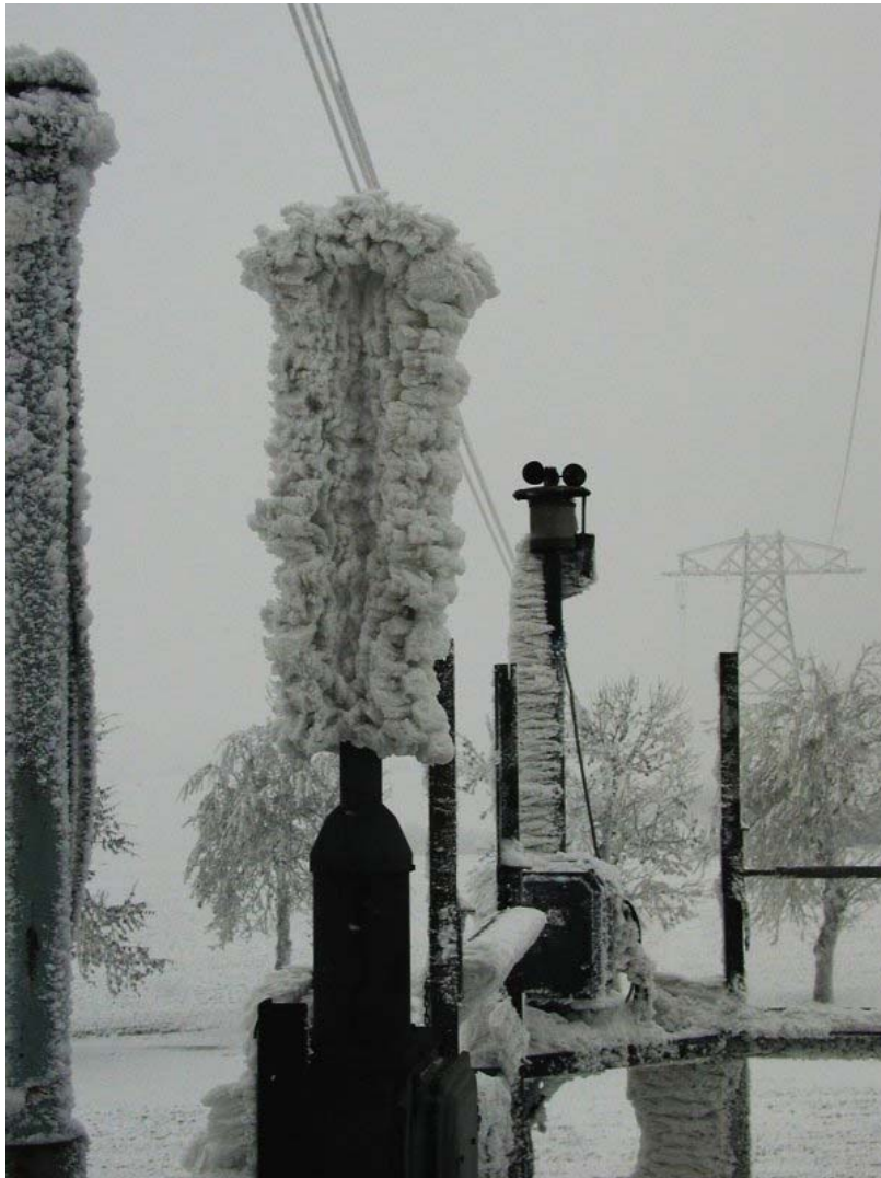
Figure A. 11 Vertical, freely rotating rod with sensor, at test site Studnice, 17.12.2004 (Photo: J.Sabata)
