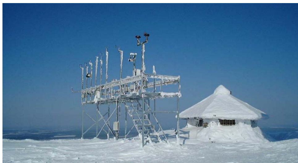
Figure A. 1 The test platform at Luosto with installed severe weather sensors.
